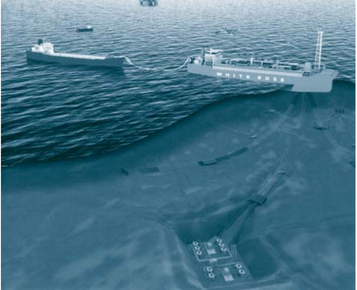
Figure 2. Offshore facilities – floating production storage and offloading system – at the Glory Hole, with cutaway showing manifold.
