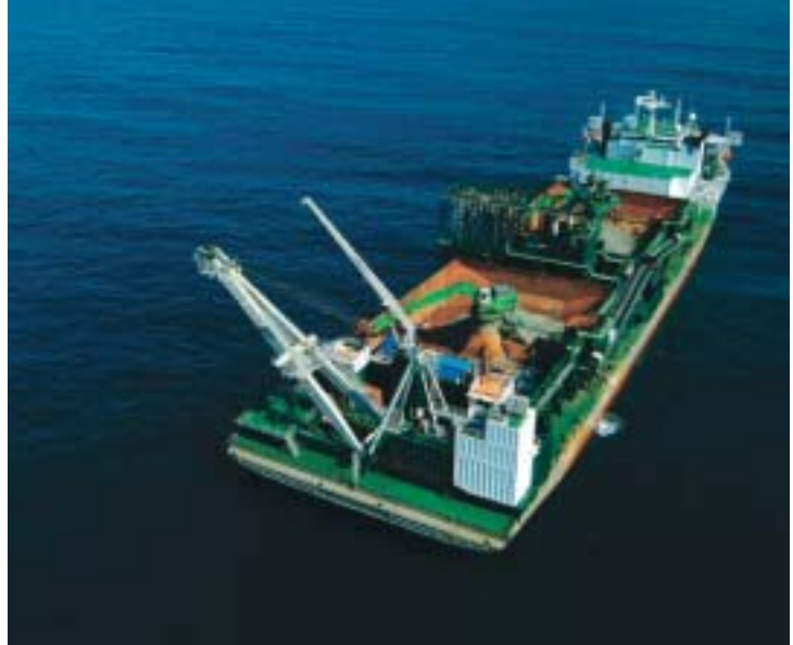
Figure 8. Grab hoisting system with A-frame for launching and recovery of grab.
