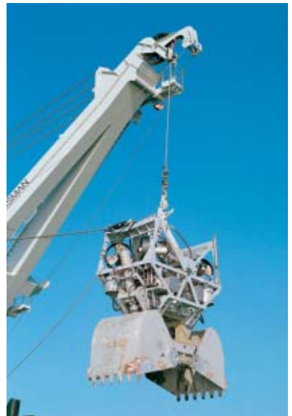
Figure 7. Assembly of clamshell and ROV suspended from A-frame.
