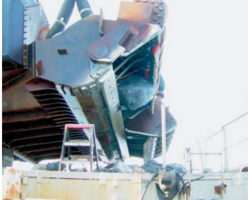
Figure 17. Draghead with boulders.
