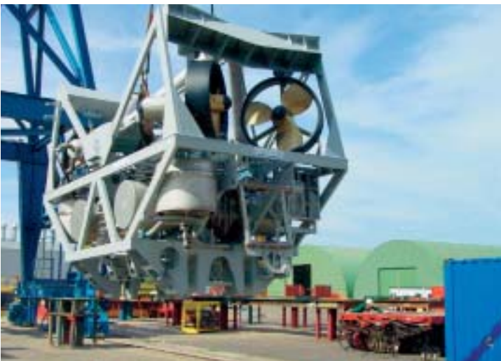
Figure 6. ROV with protective frame before assembly with clamshell.
