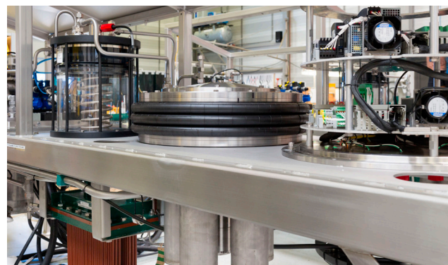
Ultralong lifetime compensator applied to subsea instrumentation
