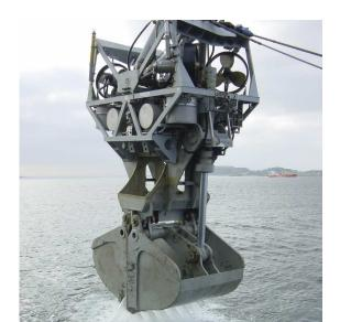
Two 250 liters heavy-duty compensators in subsea ROV grab for large stroke hydraulic cylinder compensation
