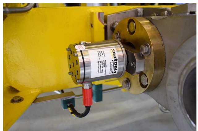
Rotax Compact sensor applied to ROV survey frame
