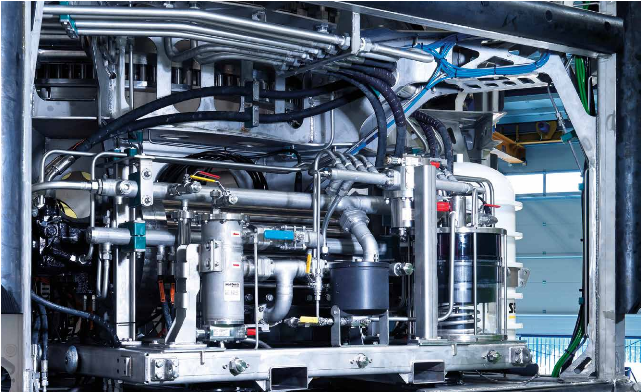
Image of a Seatools' subsea electro-hydraulic drive system.
